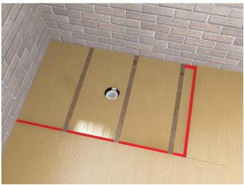
5. The sub floor can now be screwed down to the battons highlighted in blue. Note that a 160mm diameter hole has been cut to accommodate the waste trap.
