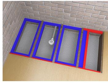
3. The battons highlighted in red have been fitted so that they are flush with the joists and support the floor. The battons highlighted in blue are sitting 18mm (floor thickness) lower than the joists to accommodate the sub-floor.
