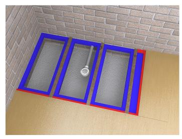
4. The extra portion of flooring that was cut away in point 2 can now be screwed back into place.
