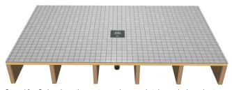
Step 10. Only when the wet area is completely sealed against leaks, can tile adhesive and tiles be fitted. Tiles should be fitted so as to maintain the drainage slope of the floor former. This completes the installation.
