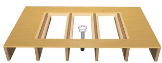
Step 4. Noggins and purlins need to be installed around all outer edges of the recess so that a sub-floor can be fitted to support the former. All adjacent flooring must be fully supported so that there is no springing between surfaces.
